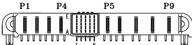
INPUT/OUTPUT CONNECTOR: P/N:molex 46437-1430
